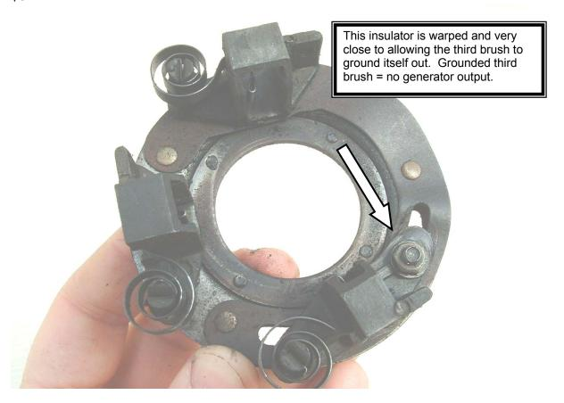
Most vendors now carry the new style insulator that is made from electrical grade fiberglass. These are excellent quality, require no cutting or fitting to install as they fit right out of the box. These are not as susceptible to cracking from over tightening the third brush like the old brittle paper ones when making a generator adjustment.
