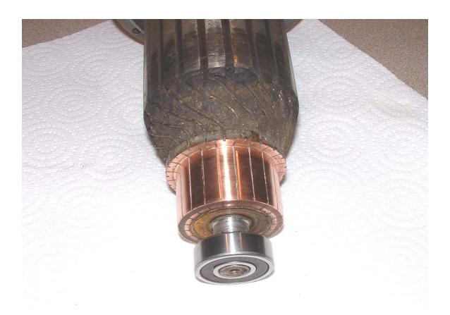
This armature is ready to install with new bearings. Truing the commutator (if needed) and polishing will ensure the new brushes make full contact after initial seating in.
