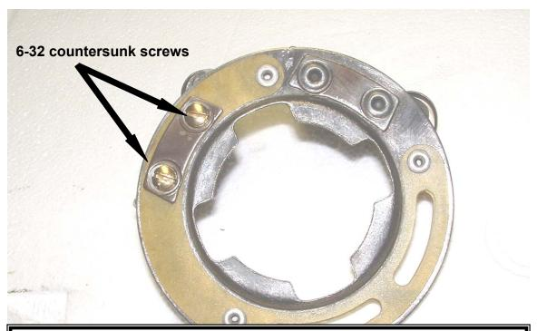
Install insulated brush and the square retaining washer that was retained after removal. If your particular brush holder didn't have this square retainer, use two thin #10 flat washers. Secure using #6-32 countersunk screws.
