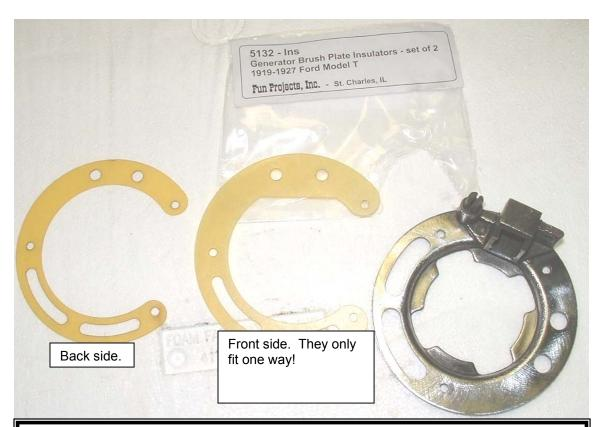
Assemble the two insulators to the brush holder as shown below. I used  $1/8 \times 1/8$  aluminum pop rivets and #6 washers. The pop rivets go in from the back, the washer goes over the end of the rivet on the front.
