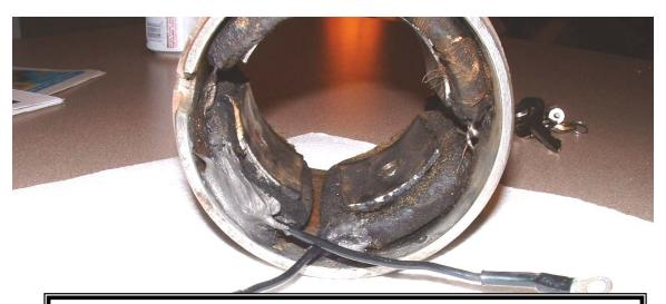
Using your ohmmeter, check to see that there is continuity between the two terminals shown. If your meter doesn't move then the fields are open and need replacing. Then, check to see that there is no continuity between either terminal and the generator housing. If the needle moves during this check the fields are shorted and need replacing. Obviously, you want to make these checks before you go through the effort of repairing the insulation.
