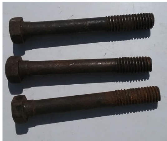
Broken head bolt. The threaded portion stayed in the block.
