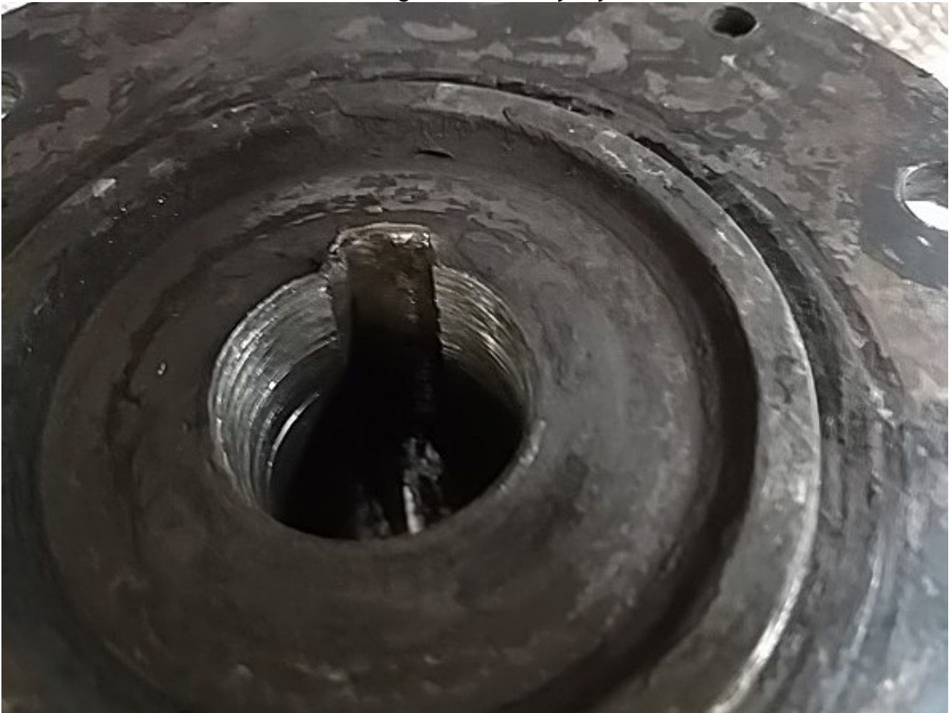
Damaged Hub and Keyway
