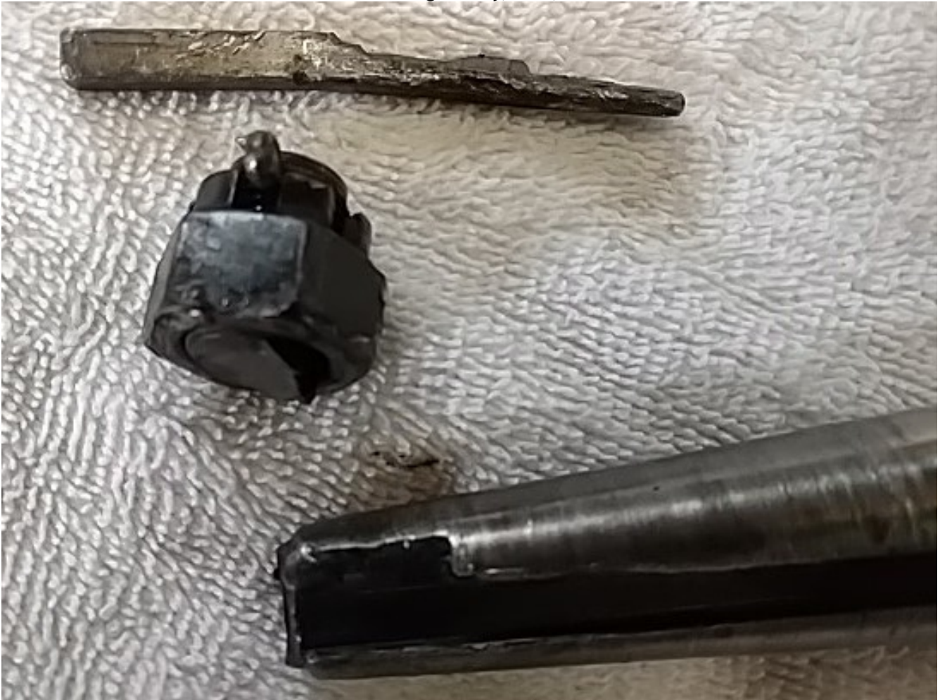
View of Damaged Key, Nut, and Axle
