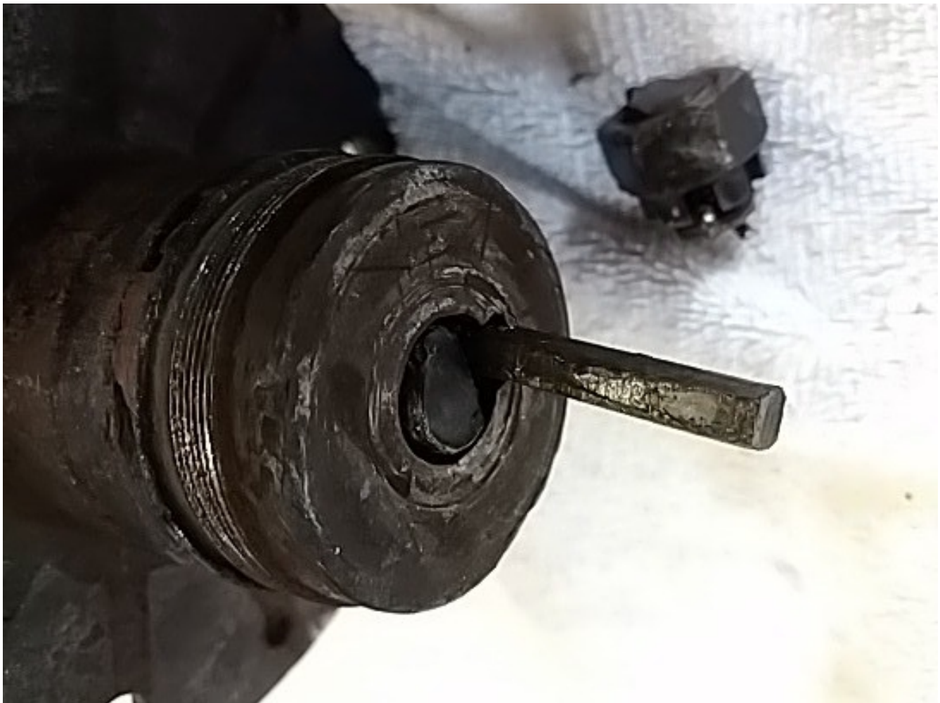
Broken Axle as Discovered
