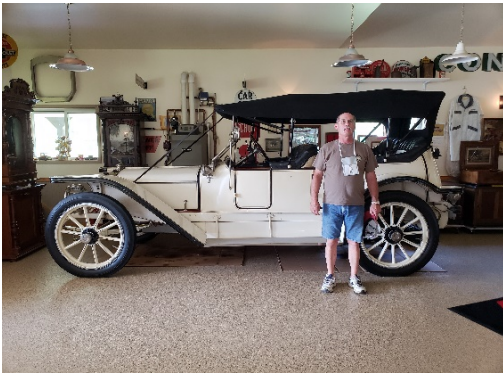
Mark stands by the only remaining 1913 Coey Flyer, body by American Traveler Body Company, with a 6-cyl, 40 hp, Herschel-Spillman motor and Stuts racing wet clutch transaxle. It originally sold for $2K and had a 10-yr warranty.
