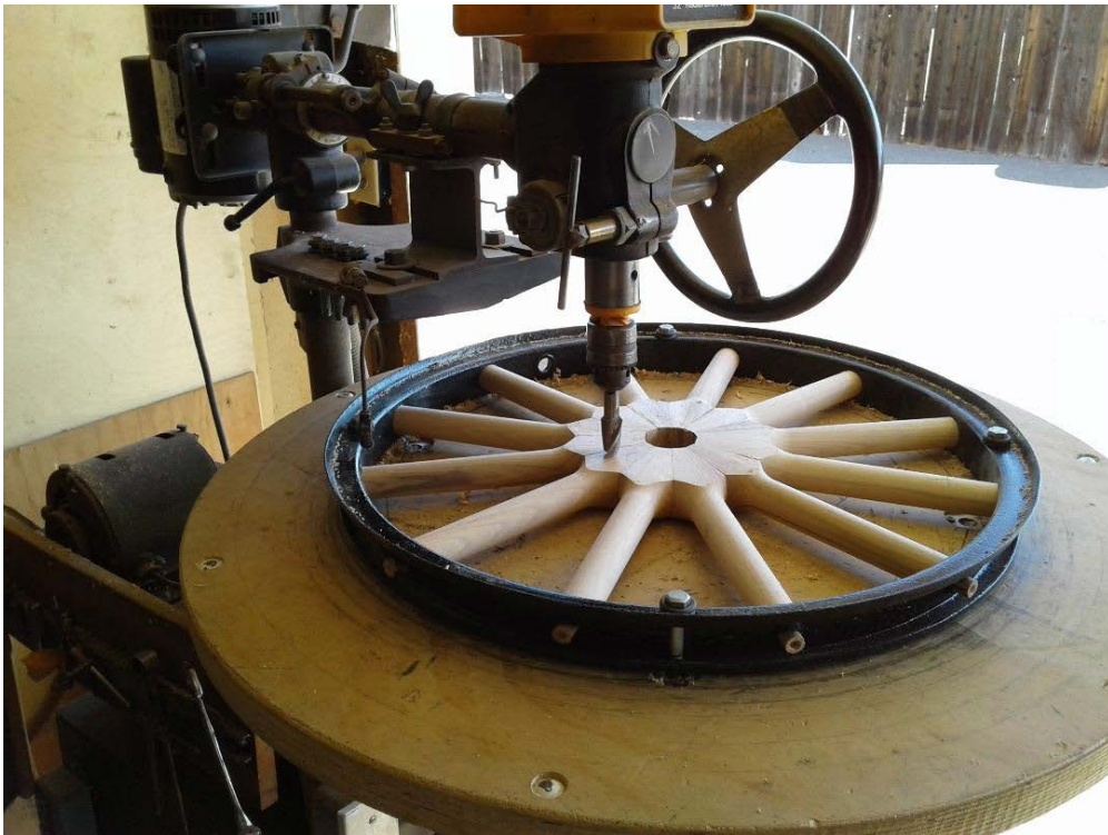
Pressed in felloes and drill for hub bolts
