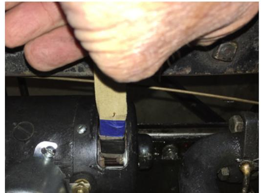
Between working on the first generator and the second, I talked to Gary Wheat and told him about my generator problem. He told me that he tried spraying WD-40 on the commutator, then then rotated the motor with the hand-crank (no power applied). He then looked at the commutator and realized that the tarnish had disappeared. He then started the motor and had charge going to the battery. **GOOD NEWS!**
