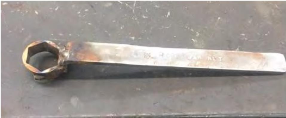
Then, I got to thinking, some folks would like a "dual" wrench- one end to loosen the nut & the other end to make the adjustment. So, this is what I did. I bought a cheapo crescent wrench at Harbor Freight and made the handle out of it, and welded it to a 15/16" socket.
