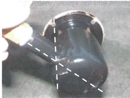
Modified Bendix Cover Showing alignment at 6 'O'clock.
