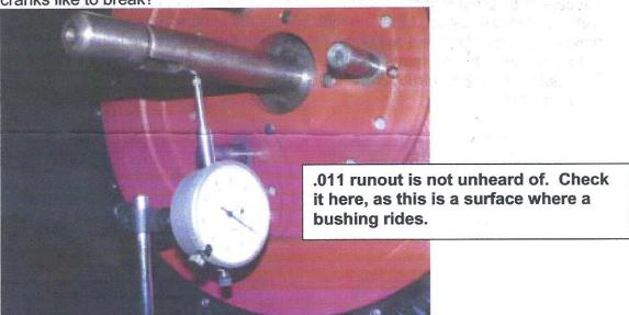
When doing this, you need to keep track of the relationship of the flywheel to the crankshaft and the transmission shaft to the flywheel. We were able to find a point where the total runout was .002, which means it was within .001 of being perfectly concentric with the crankshaft. This is within the added up clearances and should be acceptable and produce an engine that runs smoothly.
