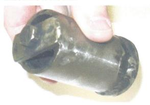
You're going to need a means to apply torque so I took a scrap bolt and a scrap piece of strap steel and drilled a hole that allows the bolt to go in. I then welded the bolt to the strap followed by welding the finished strap to the pipe. Overall, I rate this project no more than 2 cups of coffee for difficulty.
