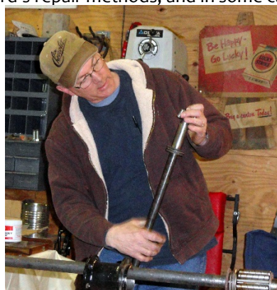
Ralph show us an often overlooked factor- worn pins that hold the steel thrust washers in place. Then, we learned how to set the lash in the ring gear and pinion.
