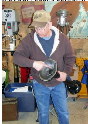
Ralph show us an often overlooked factor- worn pins that hold the steel thrust washers in place. Then, we learned how to set the lash in the ring gear and pinion.
