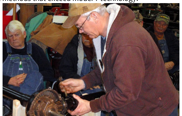
Ralph show us an often overlooked factor- worn pins that hold the steel thrust washers in place. Then, we learned how to set the lash in the ring gear and pinion.
