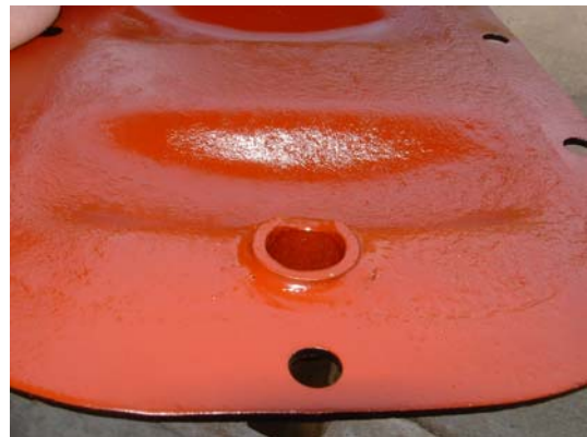
Be sure not to position the nipple so far forward as to interfere with installing the cover.
