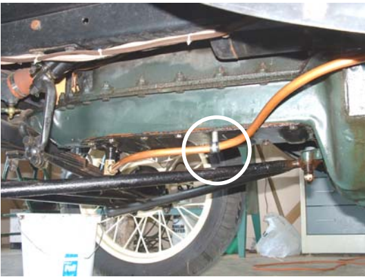
Here, I used a small bushing and a rubber lined clamp. You really need to isolate this line from vibrating. Copper has a nasty habit of breaking when allowed to vibrate.
