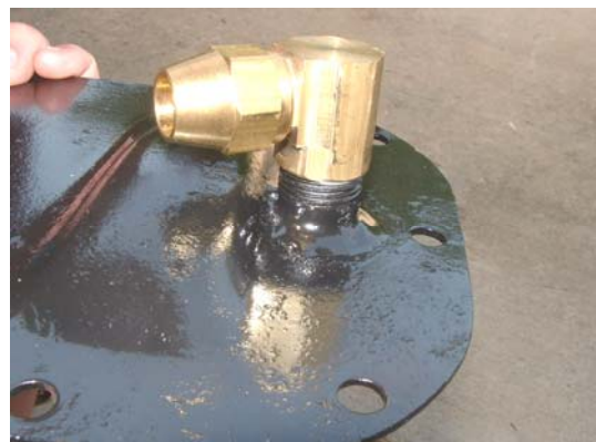
Pipe nipple needs to be long enough to prevent flare nut from touching dip cover.
