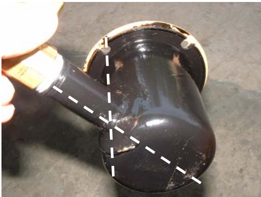
Modified Bendix Cover - showing alignment of tube at 6 'O'clock.
