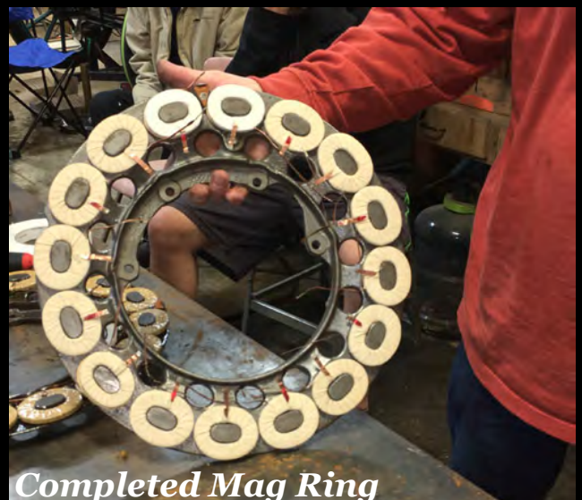
Step 6- Insulate Mag Ring
