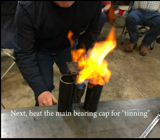
The block must be heated, then poured, and the babbitt is then "peened" into holes in the block
