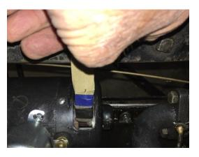
Between working on the first generator and the second, I talked to Gary Wheat and told him about my generator problem. He told me that he tried spraying WD-40 on the commutator, then then rotated the motor with the hand-Crank (no power applied). He then looked at the commutator and realized that the tarnish had disappeared. He then started the motor and had Charge going to the battery. GOOD NEWS!
