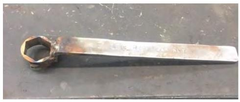
Then, I got to thinking, some folks would like a "dual" wrench- one end to loosen the nut & the other end to make the adjustment. So, this is what I did. I bought a cheapo crescent wrench at Harbor Freight and made the handle out of it, and welded it to a 15/16" socket.
