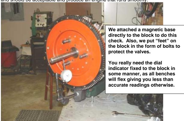
If it cannot be brought into a reasonable form of alignment, it can be corrected with a welder and lathe. Mark the high spot of the shaft when located. Then, weld a small blob on the edge of the flange. Put the shaft in the lathe and turn it cutting the weld to only leave half the total runout. Put the shaft back into the flywheel (may require a rubber mallet), bolt it back up to the crankshaft and check it again.
