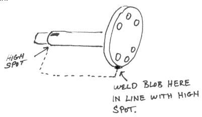
Once you have found and corrected the out of alignment condition, do yourself a favor and match mark everything! The photo below shows how I marked it using a self-striking center punch. Both the crankshaft and flywheel are marked in this photo but the main shaft is also indexed. The next one I do I will probably make
