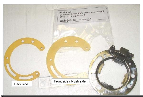
Assemble the two insulators to the brush holder as shown below. I used 1/8 X 1/8 aluminum pop rivets and #6 washers. The pop rivets go in from the back, the washer goes over the end of the rivet on the front side. To safety the pop rivets, either drive the mandrel or pin portion out or crimp the rivet with vise grips
