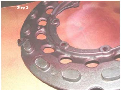
Wipe excess dye off of part. Using a rag moistened with solvent get the heavy stuff off. Don't worry about getting it all. Once the developer is applied the part will have a pink tinge to it. Cracks however will readily be evident.
