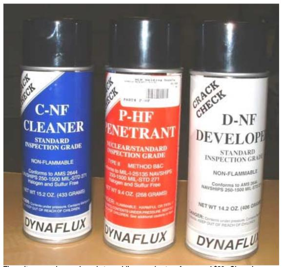
These items can be purchased at a welding supply store for around \$20. Cheap insurance before using that "good" axle shaft in your next rebuild.
