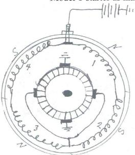
Note: In the wiring schematic you have 2 parallel paths in both the field coils and the armature.
