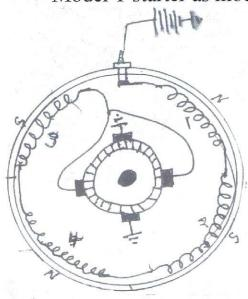
In the modified wiring the 4 field coils are in series. To keep your poles in North/South-North/South you have to swap coil 3 & 4 with each other. This wiring will drop the crank amps about 40 amps. This will result in less power from the battery and less from the starter. The result being a slightly weaker starter, about the same as if you were using an 8 volt battery on the starter like it was originally wired.
