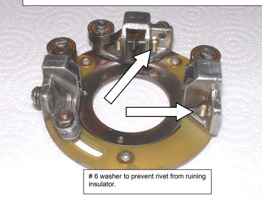
Once you have the generator put back together and have set the brushes to neutral, you can test it (sort of) even without a test bench for generators. I use my battery charger connecting the positive lead to the output terminal and ground the negative lead to the generator housing. I set my charger to six volt and once you turn it on it should run like a motor drawing four to six amps.
