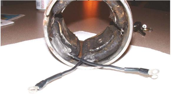
Using your ohmmeter, check to see that there is continuity between the two terminals shown. If your meter doesn't move then the fields are open and need replacing. Then, check to see that there is no continuity between either terminal and the generator housing. If the needle moves during this check the fields are shorted and need replacing. Obviously, you want to make these checks before you go through the effort of repairing the insulation.
