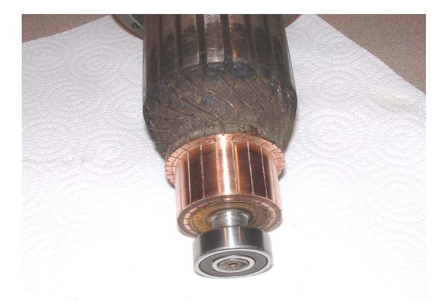
This armature is ready to install with new bearings. Truing the commutator (if needed) and polishing will ensure the new brushes make full contact after initial seating in.
