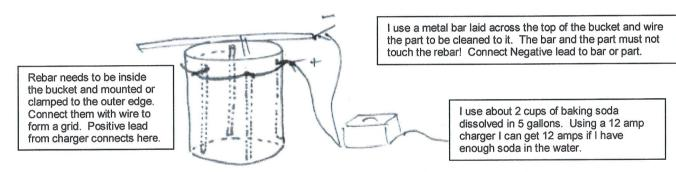
It is very important that the polarity be as shown (positive to the bucket and negative to the part). This is actually how they plate parts and what you are doing is plating the rebar with rust. Of course the rust is coming from your part. Eventually the rebar will load up and need to be replaced.
