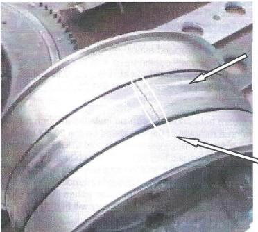
Notice this drum overheated to the point of turning blue. The owner had the band too tight and this is only 30 miles after band installation!
