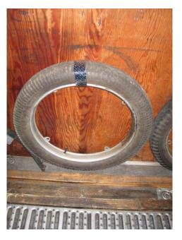
With the use of a piece of Velcro 2" wide X 18" long and a ¼" X1 ¼ fender washer, a 30 X 3 ½ Model T spare tire can be mounted inside a trailer wall. The advantage to this system is the ease of mounting and dismounting the tire repeatedly. When the spare tire is mounted resting on the trailer floor, it is secure, and an inexpensive way to store/or and transport it.
