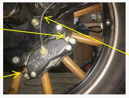
Tube that connects the caliper to the master cylinder
