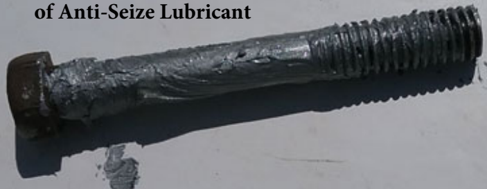
Coated with a good lathering of Anti-Seize Lubricant
