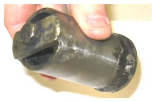
You're going to need a means to apply torque so I took a scrap bolt and a scrap piece of strap steel and drilled a hole that allows the bolt to go in. I then welded the bolt to the strap followed by welding the finished strap to the pipe. Overall, I rate this project no more than 2 cups of coffee for difficulty.
