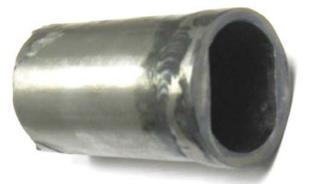
The overall length of the tool is 3 inches from end to end. If you really care about what it looks like you could chuck it in the lathe and turn off the raised portions of the weld. As you can tell, I really don't care what mine looks like.
