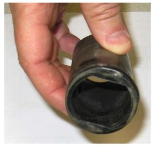
The end view shows the wheel bearing portion of the hub cap wrench welded to a scrap piece of pipe. The pipe inner diameter is slightly larger than the cam nut so clearance is perfect.
