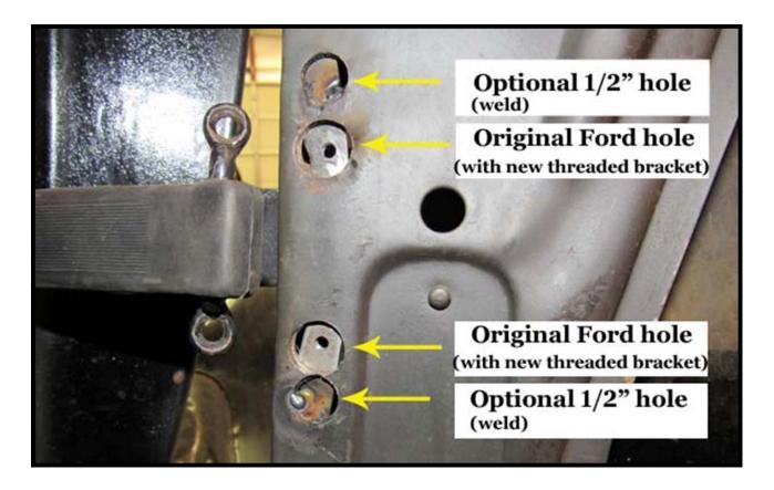
12. I used my Mig welder and lightly welded the adapter to the door at the new ½" hole that I drilled in steps 7 and 8.
