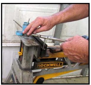
4. Once the hole is tapped, run a test screw in the newly threaded hole. The Ford book calls for a 10-32 slotted screw and the length should be at least 3/4" in order to reach the threaded hole, which will be recessed more than the standard brass adapter used by Ford.
