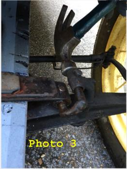
Once the bushing has been removed on spring and perch use same tool to drive in new --> bushings. Make sure you line up holes for oilers.
