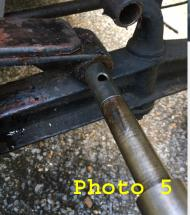
Now inserting the new shackle is a bit more challenging. I used the T jack a couple pieces scrap I had laying around and 2 rear crank shaft main bearing caps. Using the caps on either side of the axle allows the spring to be raised or lowered to get the shackle inserted.
