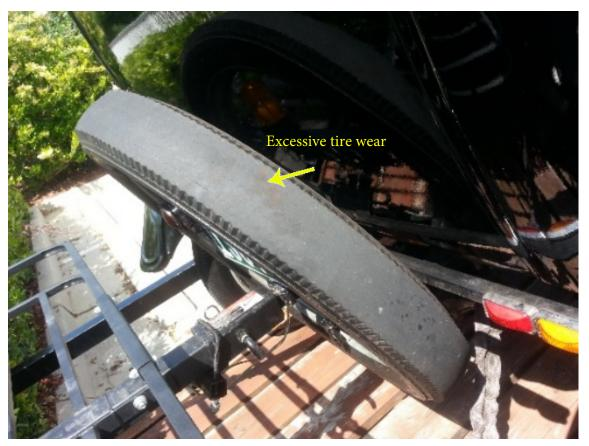
This rear tire wear anomaly developed on the Tennessee T's Spring Tour on the Natchez Trace...
