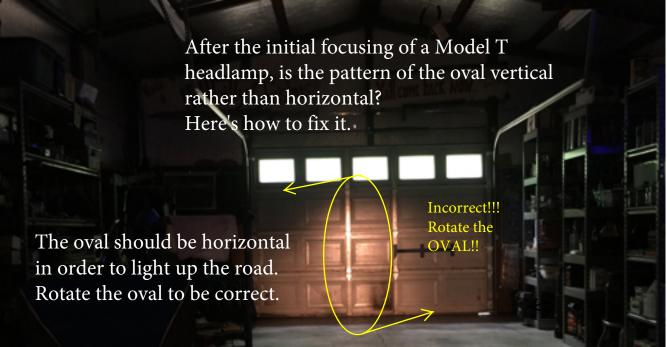
This image shows the focused oval situated vertically. This is not a good situation because it does not light up the road. Why did this situation occur? Because the vintage bulbs fit the lamp socket is such a way that the lit area aligned horizontally. Todays bulbs align the lit area vertically. The elements are made differently.
