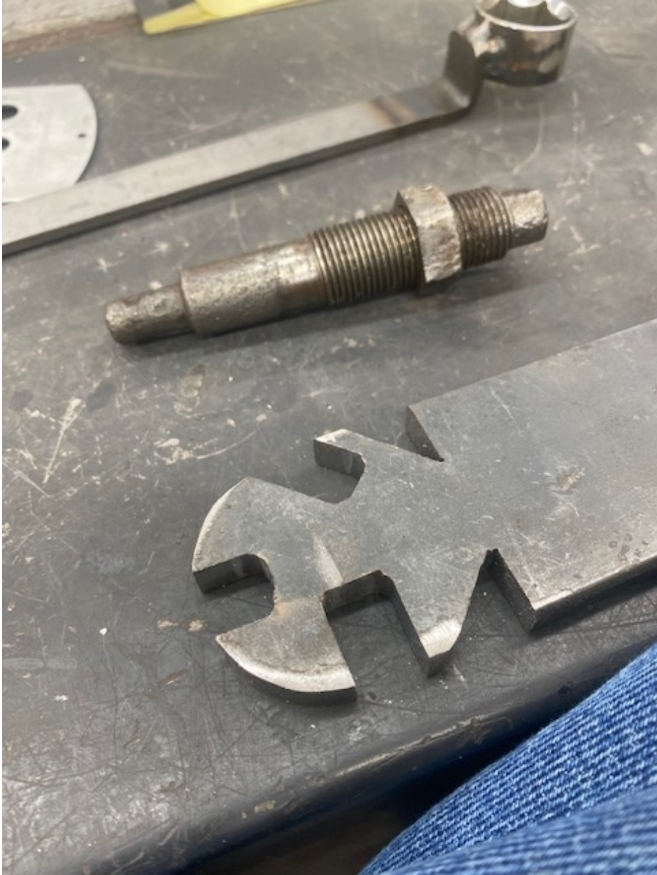
Dressing all 3 of the slots to get a good fit. This design layout allows me to put the wrench on the flats of the adjuster pin no matter what position the flats are in, from underneath the car.
