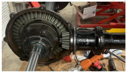
We did final assembly, safety wired, torqued and painted the entire unit as one piece and hung it back in place with our refreshed rear spring.
