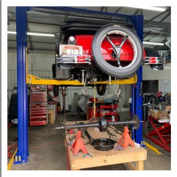
As we opened the rear end and torque tube, we were confused when we saw large chunks of soft metal in the oil we drained. Later we learned that these were parts of the babbitt bushings that the axle gears ride on. When we looked further, we saw damage from the babbitt spacer bushings crumbling and working their way through the entire rear. we decided to do a complete overhaul and rebuild the spring.
