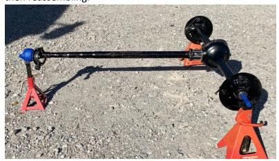
Of course, as we were putting all of the finishing touches I realized that I was about to install a damaged hub on the new axle. So, I ordered in a new hub from Lang's, watched a video on how to make a wood wheel spoke press and installed a new hub. I was amazed how well the press worked. It was astonishing!
