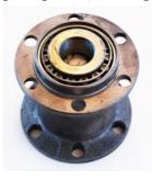
We installed the modern bearing kit into the spool that joins the driveshaft to the rear end housing and put the new pinion gear in place. Then installed the new U Joint. (One thing we learned is that the new U Joint retaining pin that you get is longer than stock. We ended up taking a bit off of it so it didn't hit the inside once it was peened over.)
