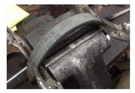
Using a hand drill with a 1/8 inch bit, you drill through from the back side, each hole for the new rivet.
