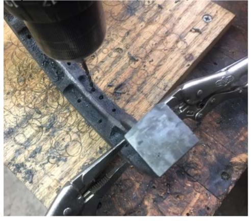
The next step is to countersink the material for the rivet heads. Because I do this operation at least once a week or more on motorcycle brake shoes, I have set up a 1/4 inch fornster drill bit with a clamp on collar to set the depth of the drill to speed up the operation.
