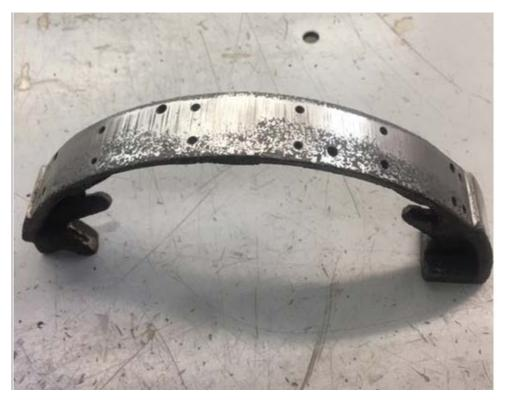
The shoe material that I use, is a modern, soft, semi flexible non asbestos lining, AF 232, that is 5/32 thick, that I buy in 20 foot rolls, from Industrial Brake and Supply. I order it in 1 1/2 inch width, but it is easily cut to any width or length desired.
