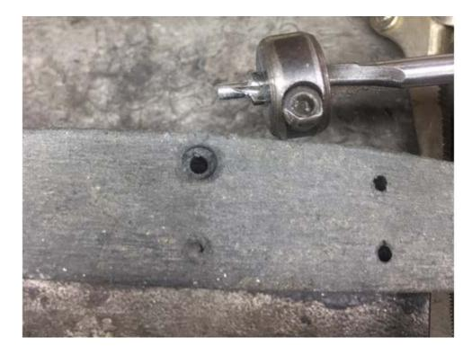
I use 3 mm copper pop rivets (almost the same as 1/8) to attach the lining to the shoes. NEVER use steel rivets, you can cut and destroy a drum, if the lining wears down to the point of contact! (You could get away with using aluminum 1/8 rivets, however) It is also critical to have a pop rivet gun, with a narrow nose, that will reach down into the recessed hole, and rest on the face of the pop rivet!
