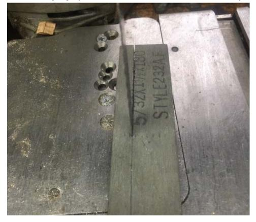
After cutting the shoe material, not only to the correct width and length, I clamped it on the steel shoe like so:
