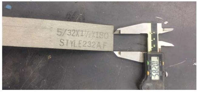
The next step is to cut the material to width. One must try to do an accurate cut, and error on the side of being slightly too wide, because this soft material is easily cut with a box cutter with a fresh
