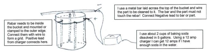
It is very important that the polarity be as shown (positive to the bucket and negative to the part). This is actually how they plate parts and what you are doing is plating the rebar with rust. Of course the rust is coming from your part. Eventually the rebar will load up and need to be replaced.
