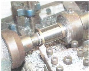
Triple gear bushing .005 tight to the case. The flange also is machined away by the amount of remaining flange on the bushing.
