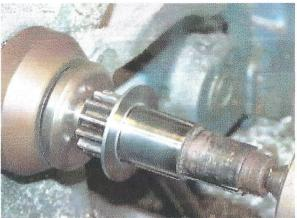
The shaft is machined allowing for the flange surface from the bushing. The bearing surface is polished smooth.
