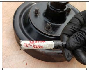
This is the Milwaukee 5/8" hole saw without a drill bit. Typical hole saws have a drill bit running thru the center.
