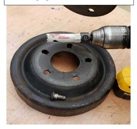
All lug studs were easily removed from this hub in a matter of minutes.
