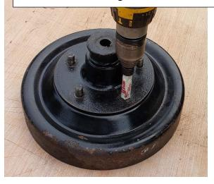
Adding a little bit of oil during the drilling process will help preserve the hole saw
