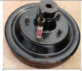
The hole saw fits directly on the swedge of the lug stud without fear of damaging the hub itself.
