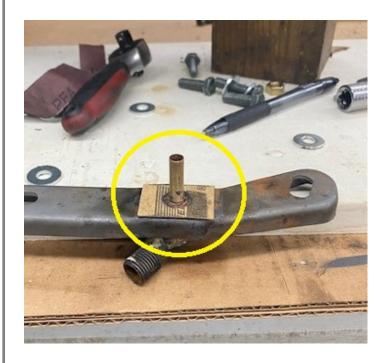
On the 1922, (which is still apart, waiting on the new engine) I had ordered a "Ford Faithful" oilier from Chaffin's to put on the car. I did not like the way the inlet for the oilier simply bolted up on the inspection cover, so I did this:
