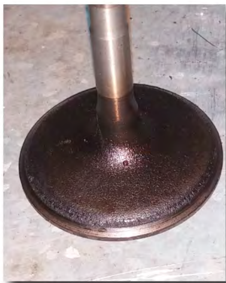
This valve is making seating properly
