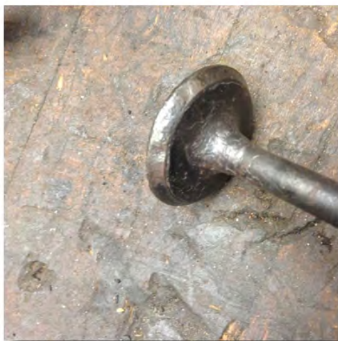
This valve is burnt and leaking
